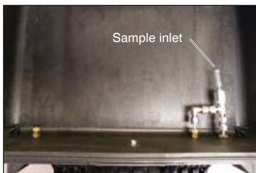
Sample inlet inside Vac-U-Chamber
