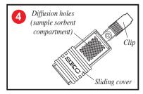
5. Stop sampling: Slide the sampler cover to the closed position (arrow and SKC visible). Write the sample stop time on the pouch label. *Important:* Measure and record ambient temperature and atmospheric pressure. Include in information sent to the laboratory.
