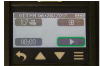
> Touch Run button in Flow Menu to run pump in constant flow.
