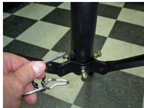
Insert pin in lower mast and tighten screws
