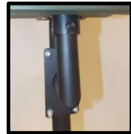
Place instrument on mounting arm. Tighten thumb screw
