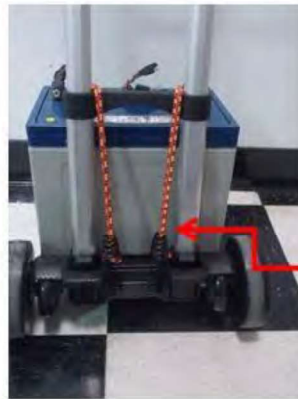
Back-up Battery Transport Cart Securing Details
