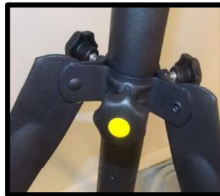
Tighten leg bracket mast thumb screws
