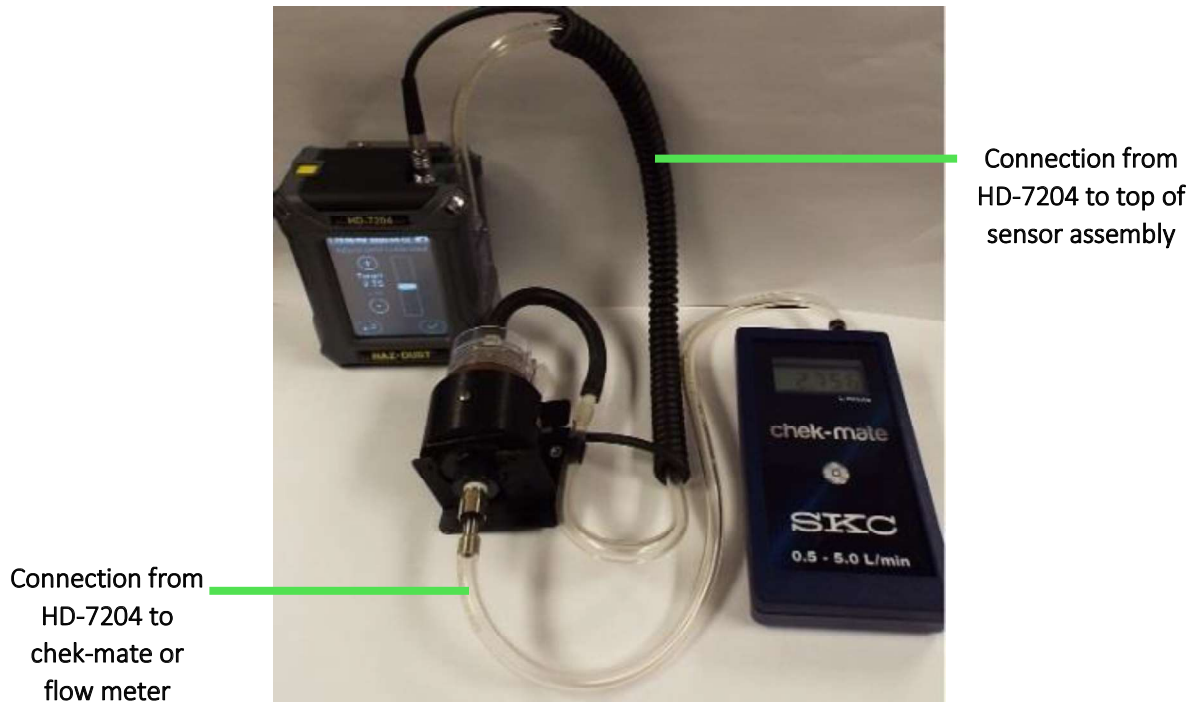
Figure 3-12. Connecting HD-7204 to SKC chek-mate
