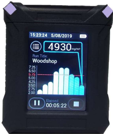
Figure 3-16. Flow Faults cause purple lights to flash
