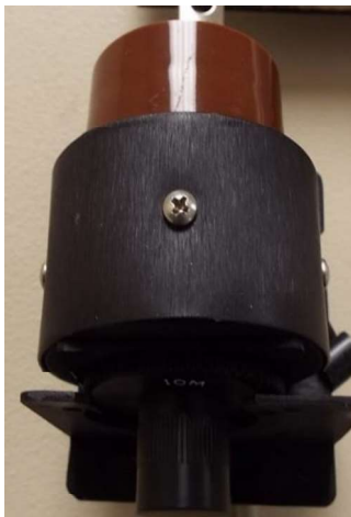
Figure 3-15. CS-7204 being inserted into HD-7204 sensor
