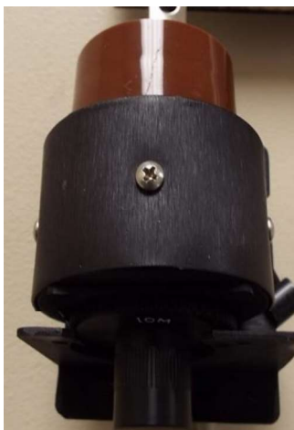
Figure 5-1. CS-7204 being inserted into HD-7204 sensor
