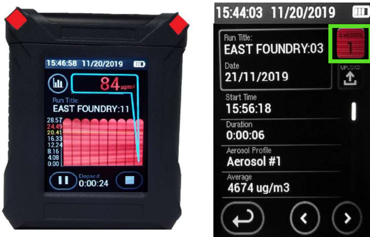
Figure 3-17. Battery Faults cause red lights to flash
