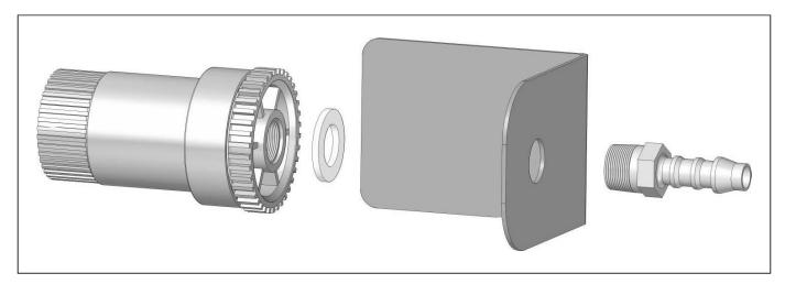
Screw the threaded hole on the asbestos sampling head onto the male thread at the top of the sampling mast.
