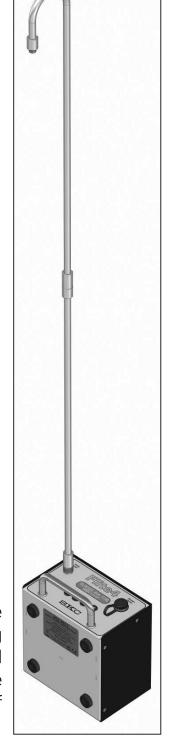
5. Note - If the full 1 metre mast height is not required, use only the mast section(s) required to achieve the necessary height.
