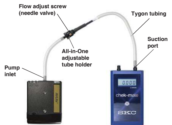
Calibration train with All-in-One connected to AirLite
