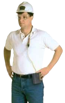
Clip tube holder to worker and pump to belt.
