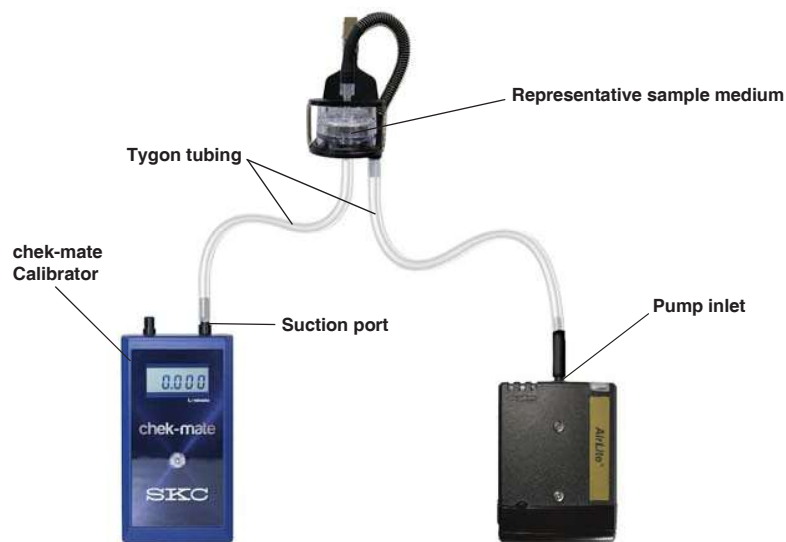
Calibration train with filter cassette
