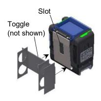
2. Rotate the holder 90 degrees so that the toggle catches securely inside either side of the slot and the bottom plate of theholder is parallel with the bottom of the pump.
