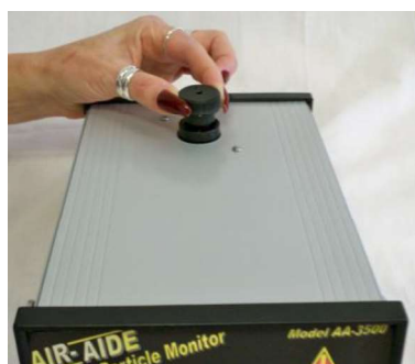
Figure 3-8. Installing the span calibration insert into the Air-Aide Monitor
