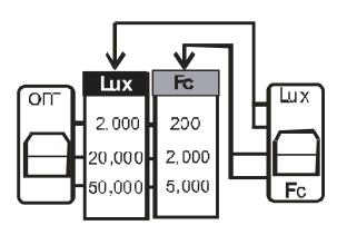
Example: If a measurement on the 5000 Fc range displays 350 the actual measured value is:  $350 \times 10 = 3500 \text{ Fc}$ .
