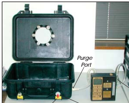
Figure 4. Universal Series Sampler connected to a small Vac-U-Chamber for purging a bag or purging the sample line
